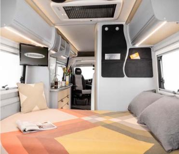
Redefining storage, the east/ west double bed is built on gas struts, and when in its upright position, provides walk through access, space to stow your longer, bulkier adventure equipment, additional living space and extra sitting area.
